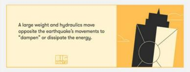
Another damping method is pendulum power, used primarily in skyscrapers. Engineers suspend a large ball with steel cables with a system of hydraulics at the top of the building. When the building begins the sway, the ball acts as a pendulum and moves in the opposite direction to stabilize the direction. Like damping,
