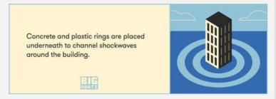
Instead of just counteracting forces, researchers are experimenting with ways buildings can deflect and reroute the energy from earthquakes altogether. Dubbed the "seismic invisibility cloak", this innovation involves creating a cloak of 100 concentric plastic and concrete rings in and burying it at least three feet beneath the foundation of the building.
