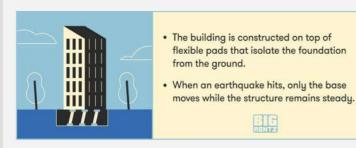
One way to resist ground forces is to "lift" the building's foundation above the earth. Base isolation involves constructing a building on top of flexible pads made of steel, rubber, and lead. When the base moves during the earthquake, the isolators vibrate while the structure itself remains steady. This effectively helps to absorb seismic waves and prevent them from traveling through a building.
