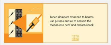
The first method involves placing dampers at each level of a building between a column and beam. Each damper consists of piston heads inside a cylinder filled with silicone oil. When an earthquake occurs, the building transfers the vibration energy into the pistons, pushes against the oil. The energy is transformed into heat, dissipating the force of the vibrations.
