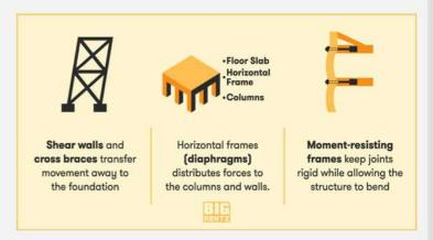
To withstand collapse, buildings need to redistribute the forces that travel through them during a seismic event. Shear walls, cross braces, diaphragms, and moment-resisting frames are central to reinforcing a building.
